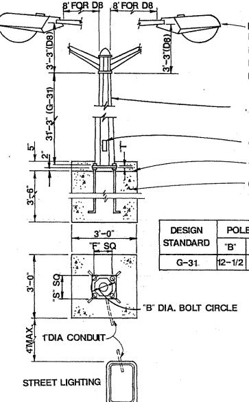
LUMINAIRE AS MANUFACTURED BY GENERAL ELECTRIC CO. OR APPROVED EQUAL WITH RECEPTACLE FOR EXTERNAL MOUNTED PHOTOELECTRIC CELL \*LUMINAIRE SHALL BE EQUAL TO GE#C724N806 W/#C402G600 PHOTOELECTRIC CELL & 250W HPS LAMP.
