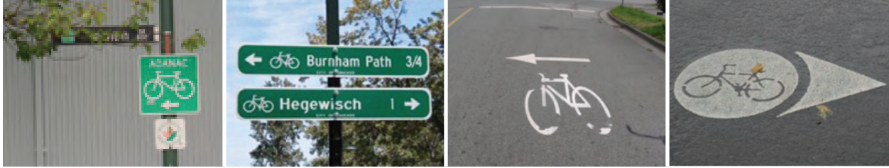
FIGURE 10.24 Examples of directional signage (left two images) and pavement markings (right two images).
