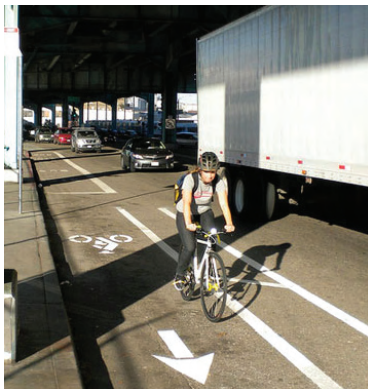
FIGURE 10.10 Buffered bicycle lane.
