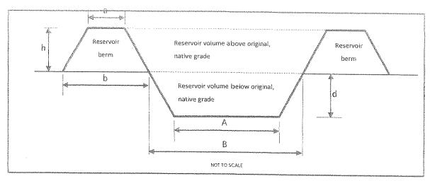
Figure 5. Cross Section of Typical Reservoir and Surrounding Berm.
