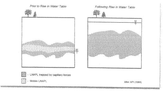
Figure 4. Effect of rising water table on LNAPL distribution in porous medium.
