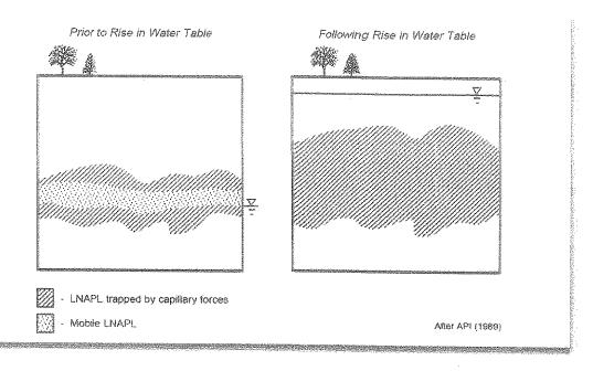
Figure 4. Effect of rising water table on LNAPL distribution in porous medium.
