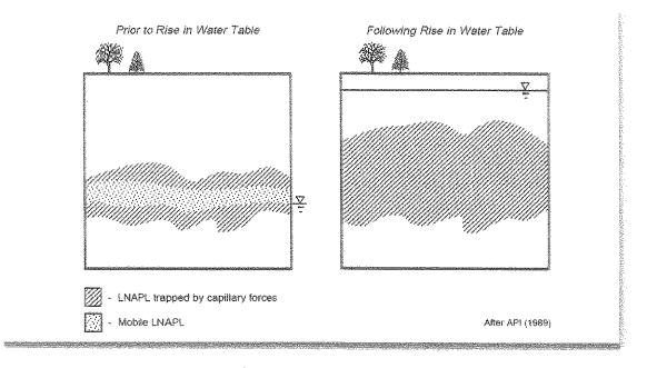
Figure 4. Effect of rising water table on LNAPL distribution in porous medium.
