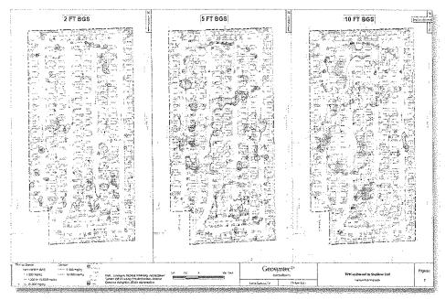
Figure 3. TPH as diesel in shallow soil.
