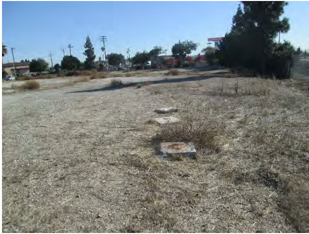
13. Typical groundwater monitoring wells.
