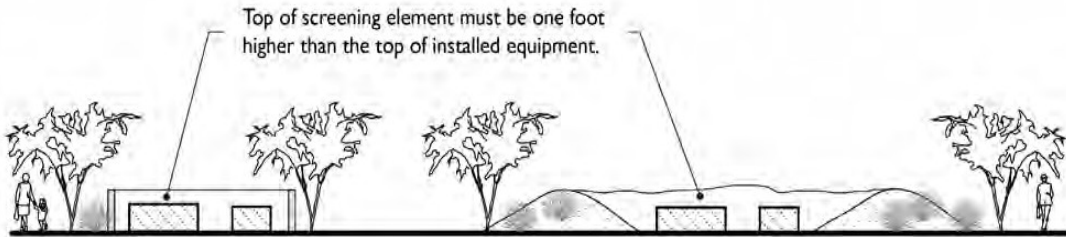
FIGURE 9311.7-B: SCREENING OF GROUND-MOUNTED EQUIPMENT
