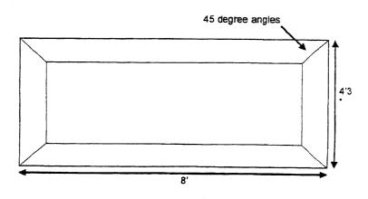
shape of the bed. See the comer diagram below.] The 2"x6"x8" lumber will remain this length. Now cut 45 degree angles in the 8' and 4'3" bench pieces so that they fit together as shown above.
