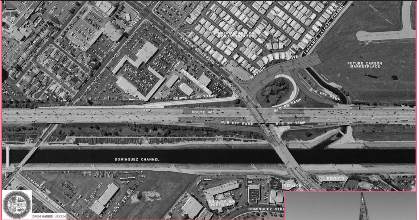
**C**onstruction on the Avalon Boulevard Interchange on the I-405 started on August 2010 to add a new southbound on-ramp on the 405 and a bridge to access the Boulevards project. The project scope also involves realigning and improving existing ramps, widening of the 213th Street Bridge, building eight retaining walls and a sound wall, construction of Lenardo Drive, and widening of Avalon Boulevard. The \$19.3 million project is expected to be completed in December 2011.
