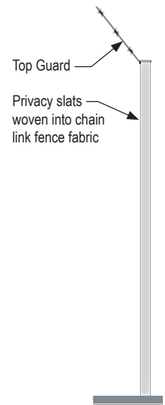
Figure 5–1: Distribution Facility Perimeter Fence Typical Section
