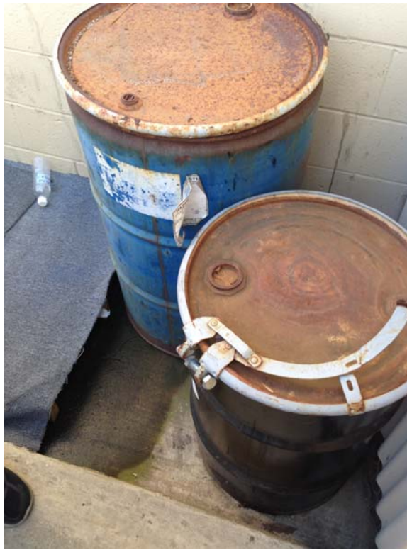
Waste PCE storage area in the rear of Happy Cleaners unit; visible leaks, possible PCE 21609-21635 Avalon Blvd. & 645-655 E Carson St.
