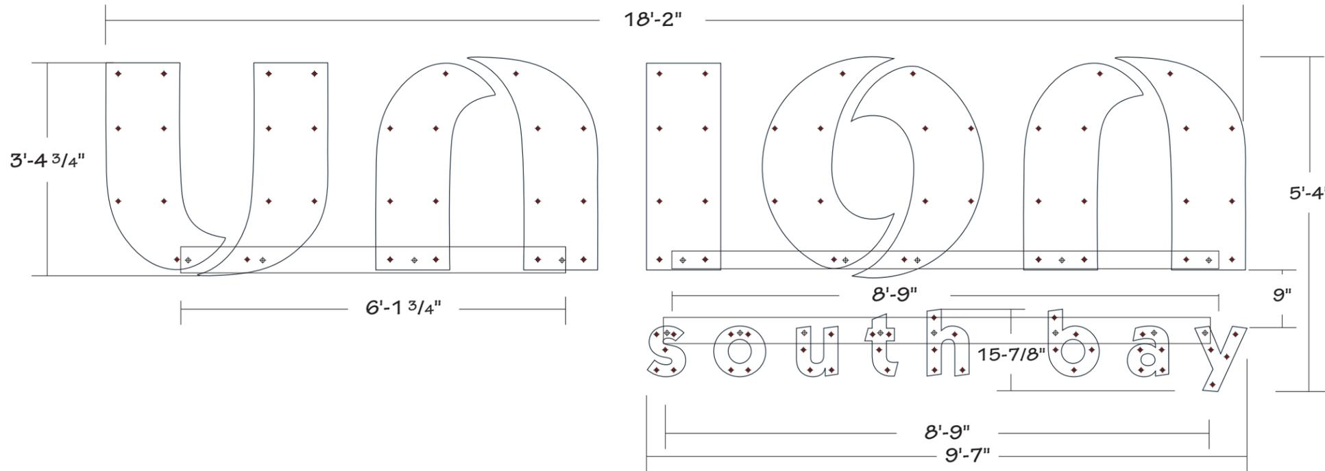
1. Ensure wall location for sign is correct. Position paper pattern in correct location. Ensure pattern is level, tight, and taped every 6" to prevent slack. Ensure that electrical supply is in place.
