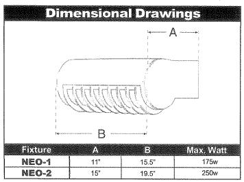
The **NEON** is a recessed wall mount luminaire, designed for illuminating pedestrian pathways, stairwells, indoor parking garages, and other general area lighting applications.
