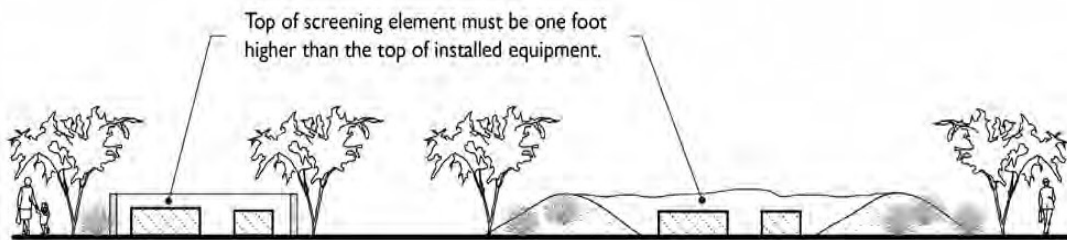
FIGURE 93 I 1.7-B: SCREENING OF GROUND-MOUNTED EQUIPMENT
