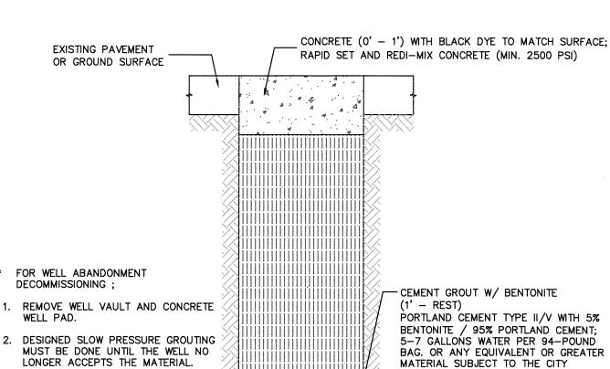
CEMENT GROUT W/ BENTONITE (1' - REST) PORTLAND CEMENT TYPE II/V WITH 5% BENTONITE / 95% PORTLAND CEMENT; 5-7 GALLONS WATER PER 94-POUND BAG. OR ANY EQUIVALENT OR GREATER MATERIAL SUBJECT TO THE CITY ENGINEER'S APPROVAL.
