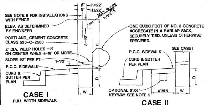
SLOPE 3:1 OR AS **DETERMINED BY ENGINEER**  PARTIAL WIDTH SIDEWALK HOUSE WALK "a"
