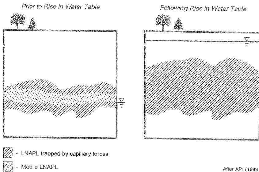
Figure 4. Effect of rising water table on LNAPL distribution in porous medium.
