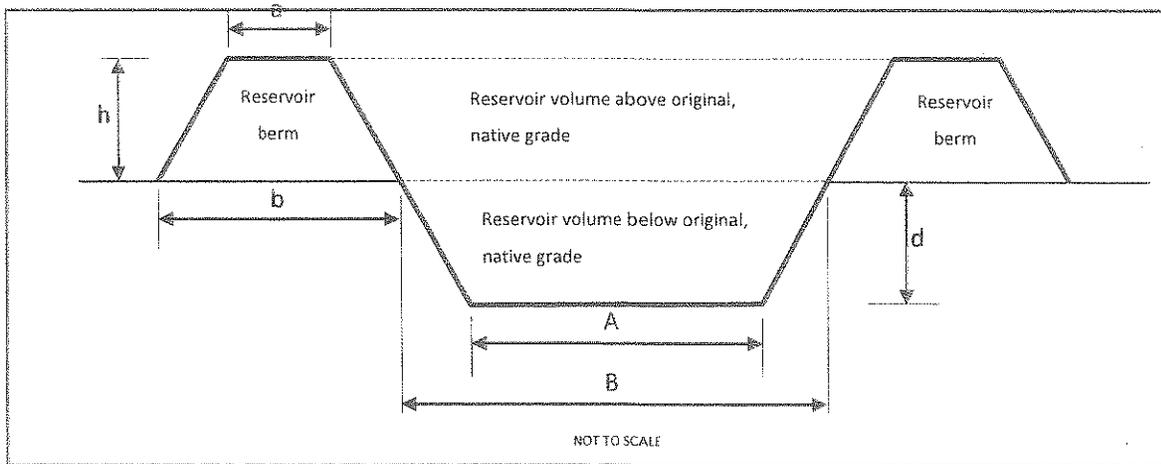
Figure 5. Cross Section of Typical Reservoir and Surrounding Berm.
