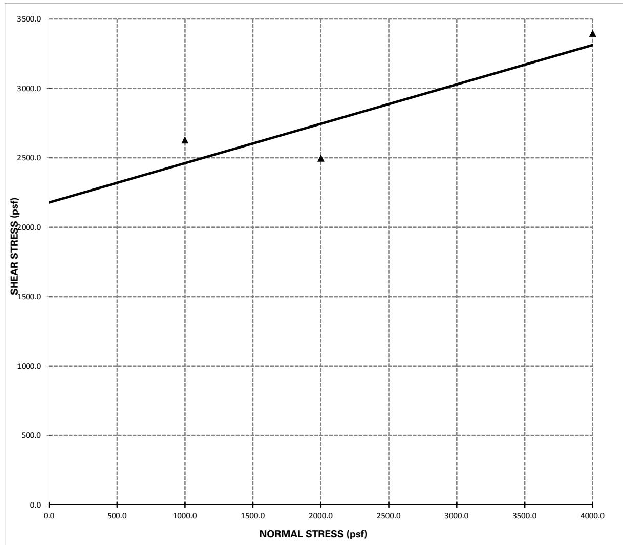
**Shear Strength:**  $\Phi = 15.8^\circ$  ;  $C = 2178.0 \text{ psf}$
