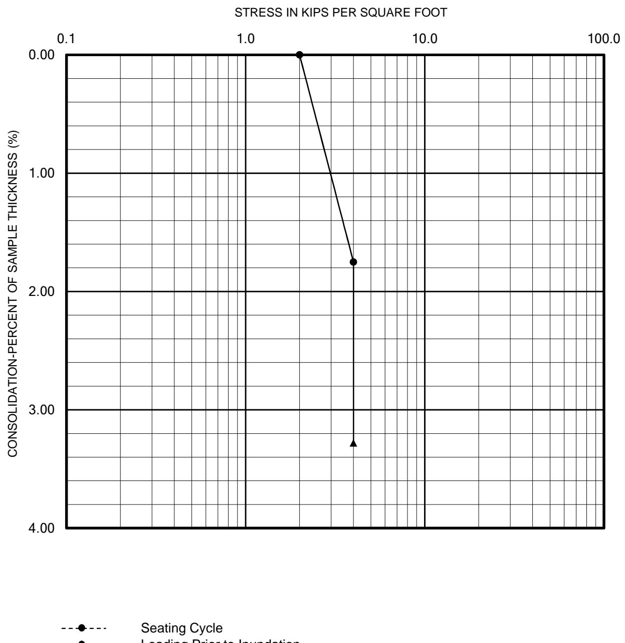
PERFORMED IN GENERAL ACCORDANCE WITH ASTM D 4546
