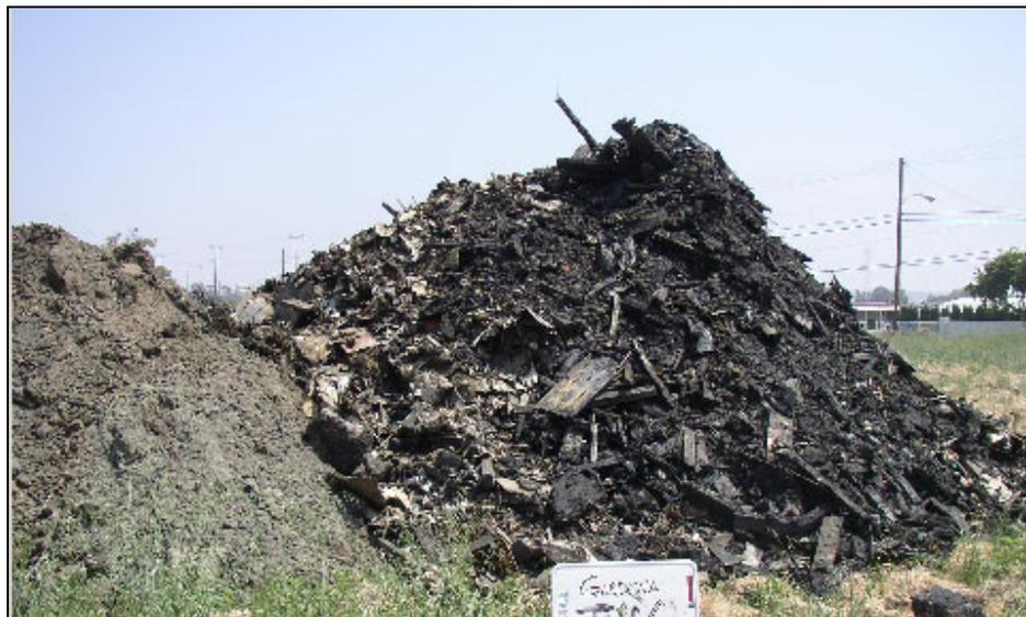
Figure 2. Typical soil cap material (left) and waste debris (right)
