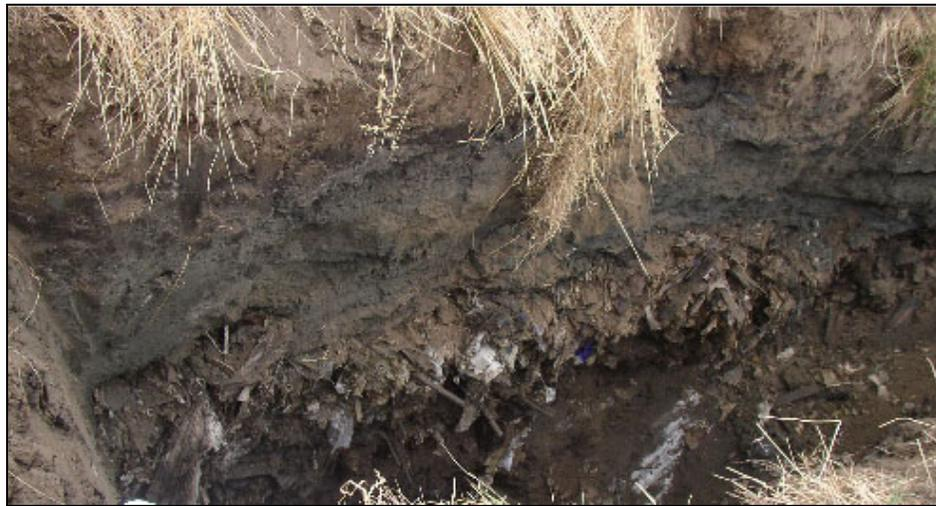
Figure 1. Typical Trench profile (soil cap material overlying waste debris)
