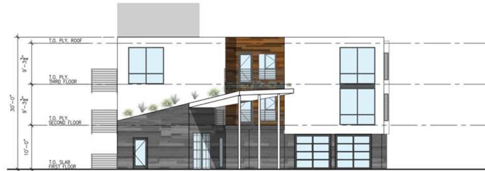
BUILDING TYPE-A WEST ELEVATION SCALE: 1/8"= 1'-0"
