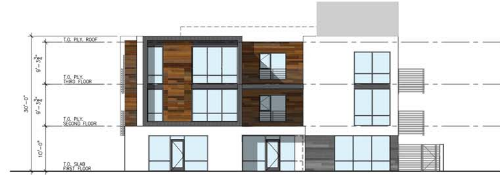
BUILDING TYPE-A EAST ELEVATION SCALE: 1/8"= 1'-0"
