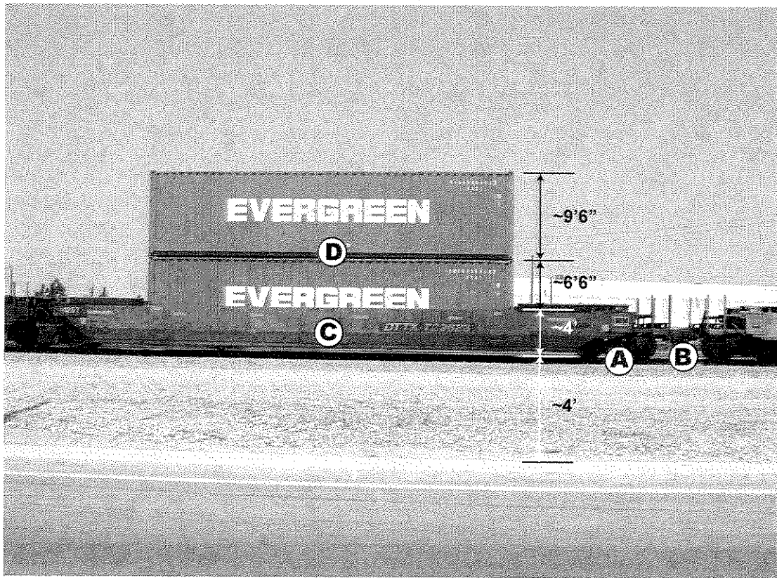
Figure 2: Noise Source Locations for Container Flatcar
